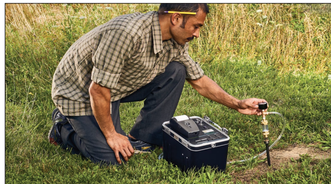
The Soil Gas Probe Accessory - for soil gas sampling
