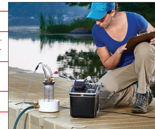
The RAD AQUA Accessory for monitoring radon in water
